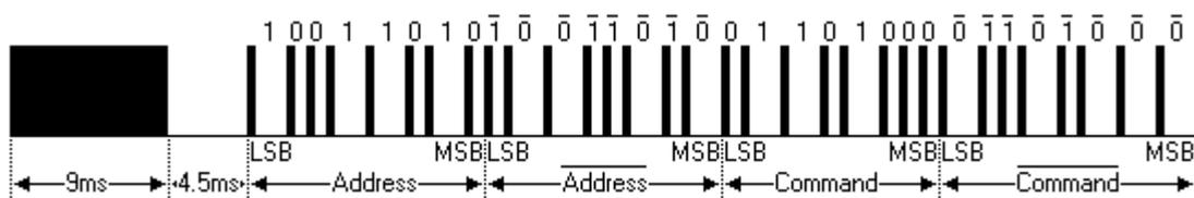
The picture above shows a typical pulse train of the NEC protocol. With this
